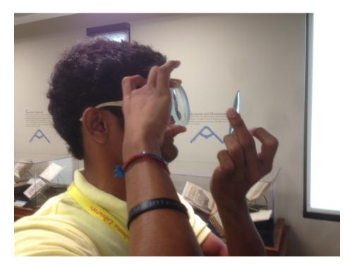
3. Position the two lenses in a line at eye-level, with the flat sides facing toward each other. Try to focus on an object a few feet away. Hold the plano-concave lens close to your eye, and the plano-convex lens a few inches farther away. *Is the object right-side-up or up-side-down?*
