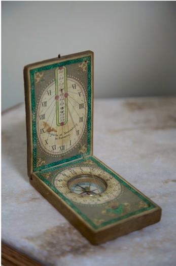
A sundial consists of a **gnomon**, which casts the Sun's shadow, and a **dial** on which the shadow indicates the time. On a **pocket sundial** by David Beringer (c. 1760), the gnomon is a short length of string which casts a shadow on the vertical dial. The horizontal compass enables the pocket dial to be positioned facing due south. **Polyhedral sundials** have a gnomon on every face, with dials aligned to tell the same time on each face.
