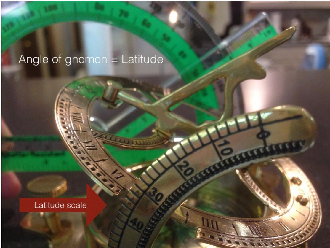
3. Tilt the dial so that it indicates the **current latitude (35°N)** on the latitude scale. When moved into this position, the angle between the horizontal platform and the gnomon itself should be equal to one's latitude on Earth. The latitude of Norman is 35°N.
