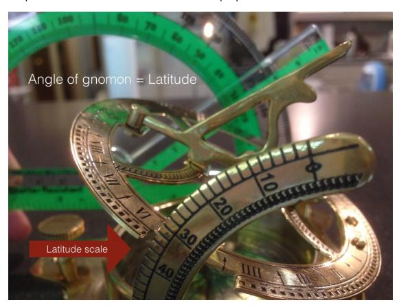
3. Tilt the dial so that it indicates the **current latitude (35°N)** on the latitude scale. When moved into this position, the angle between the horizontal platform and the gnomon itself should be equal to one's latitude on Earth. The latitude of Norman is 35°N.
